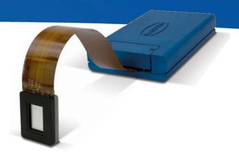
The analog ERIS Spatial Light Modulator shows extreme phase stability, low latency and the display architecture allows low crosstalk LCOS-cell designs.
