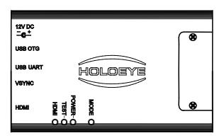
The PLUTO-2.1 driver features a dual-core ARM® Cortex $^{TM}$ -A9 processor which includes on-chip memory. This enables the user to program additional functionality which is directly processed on the SLM device.
