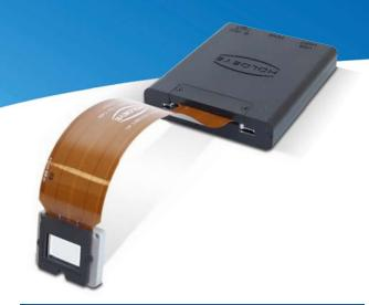
The LETO Spatial Light Modulator is our fast SLM platform with high band width. The SLM is capable of color sequential operation.
