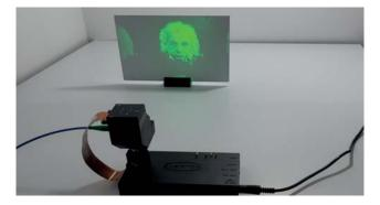
The diffractive approach uning a phase SLM is fairly simple as it only requires a linearly polarized light source and the SLM itself. However, as diffraction angles are limited (dependent on pixel size of the used SLM) it might be necessary to use additional optics to magnify the output image.
