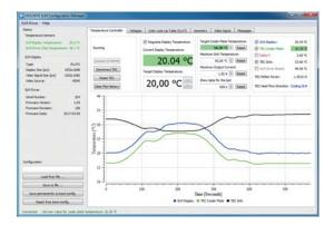
All HOLOEYE LCOS SLM displays feature an integrated temperature sensor. A USB connection is used to connect the temperature control unit to the PC.
