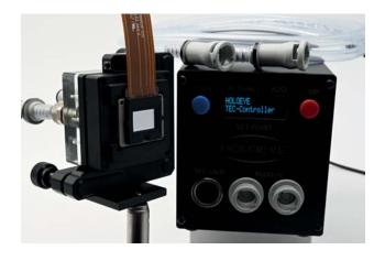
The up-to date display versions of all these SLM platforms use a standardized display packaging with a ceramic stiffener / back plate with excellent thermal conductivity. The displays can be mounted using the integrated magnets or by screws if required.
