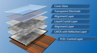
LCOS technology is a powerful combination of two well-developed technologies: IC/CMOS and Liquid Crystal (LC). LCOS has a significant advantage in high-end projection applications due to the maturity and potential of both IC/CMOS and LC technologies.
