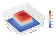
Diffractive Diffusers can be best used with VCSEL arrays, because they consist of many individual incoherent laser emitters. As a result, the angular far field diffracted light distribution is much less
