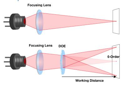
Laser diodes are the most common light source to be used with diffractive optical elements, but other laser light sources may also be used.
