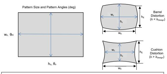
$\theta_H$ = horizontal angle,  $\theta_V$ = vertical angle,  $h_C$ = center height,  $w_C$ = center width,  $h_E$ = edge height,  $w_E$ = edge width
