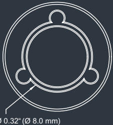
Thorlabs 8 mm steel lens adapter
