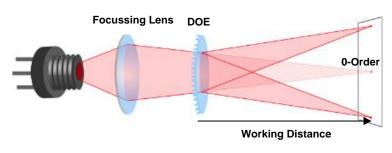
Laser diodes are the most common light source to be used with diffractive optical elements, but other laser light sources may also be used.
