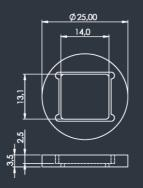
25 mm anodized aluminum mount with 14.0 x 13.1 mm clear aperture
