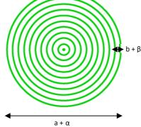
Pattern size and pattern angles and the intensity in the undiffracted central spot ('zero order intensity', see reverse page) will vary most with the wavelength. Within the recommended wavelength range, the element shows the lowest intensity in the central spot.
